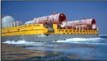
On the other side of the world, the 250 tonne payload "Sea Pearl", designed by Mackace Ltd. (Mackley Air Cushion Equipment) in the U.K., was at that time the largest hover barge in the world. Built in the mid-70s near the Mina Zayed (Zayed Port), Abu Dhabi's oldest commercial port to meet Lloyds regulations, the barge was capable of handling 2 – 3m wave heights at sea. "Sea Pearl" became the workhorse that facilitated the United Arab Emirates' expansion of their offshore oil and gas
